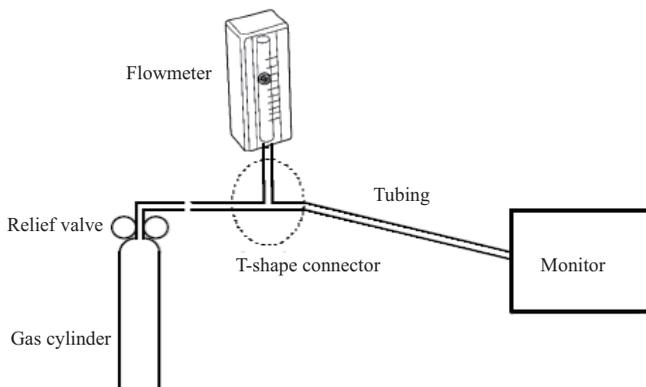
6. Turn on and adjust the relief valve to make the flowmeter reads within 10-50 mL/min and keeps stable as well.
