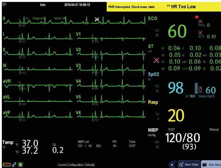
There are a total of 12 ECG waves and 1 rhythm wave displayed on the screen. The rhythm lead is consistent with what is set for ECG1 before entering the 12-lead ECG screen.
