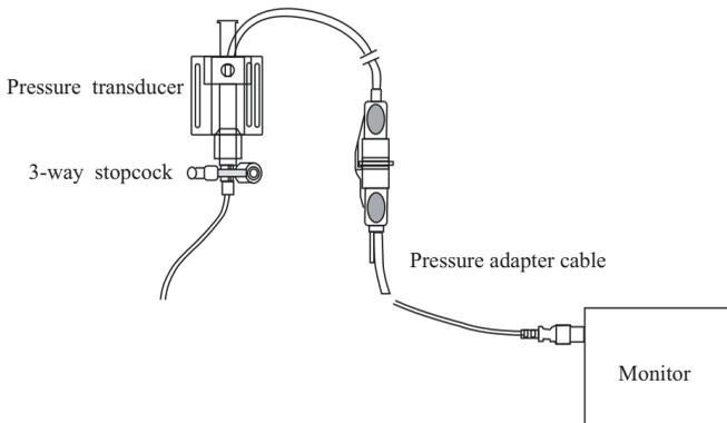
2. Vent the transducer to the atmospheric pressure by turning on the stopcock to the air.
