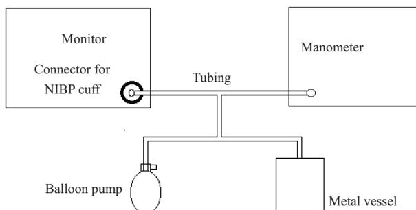
2. Before inflation, check that the reading of the manometer should be 0. If not, open the valve of the balloon pump to let the whole airway open to the atmosphere. Close the valve of the balloon pump after the reading is 0.
