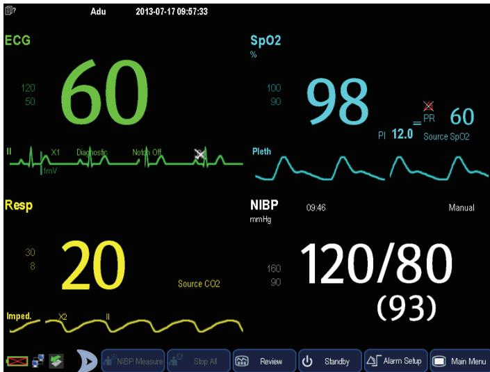
You can select your desired parameters to display in this screen: select the [Screens] QuickKey→[Big Numerics Screen Setup] and then select the parameters you want. For parameters having a waveform, the waveform will also be displayed.
